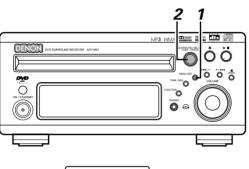
With the function set to DVD, press the STATUS button of the remote control for at least 2 seconds.
